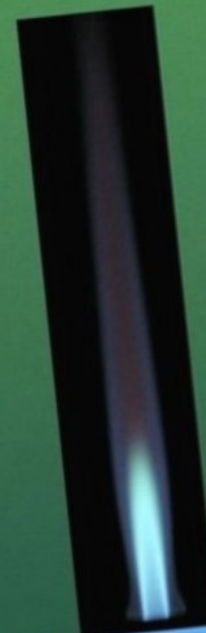
Non-Luminous Flame It is formed when the air-hole is closed
